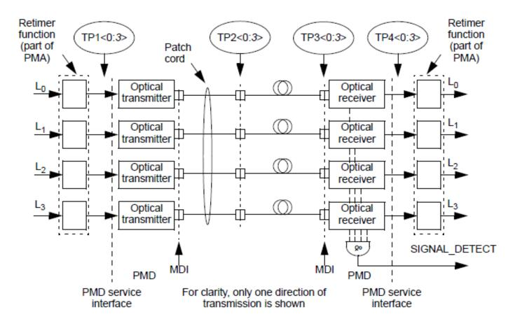
• TP1 and TP4, shown here for illustration only, represent the start and end of link budget calculations. They may not be accessible points for measurements, nor are they intended as reference points for specifications
