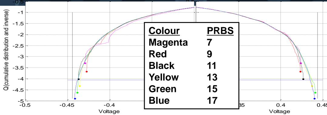
PRBS7 to PRBS11 are too short to find the in-service peak-to-peak voltage with user data not a test pattern
