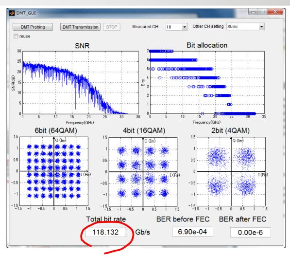
Channel bandwidth was limited to 10GHz due to long PCB traces on DAC & ADC evaluation boards.
