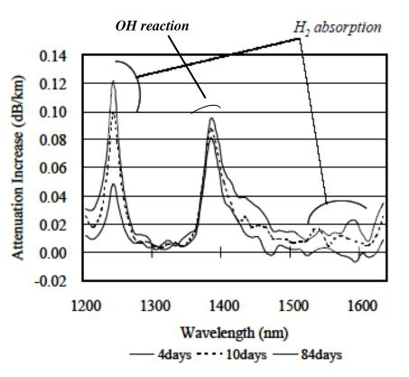
Ref: M. Shimizu et. al, "Hydrogen Aging Tests for Optical Fibers", *IWCS Proceedings*, p. 219-223, (2001)
