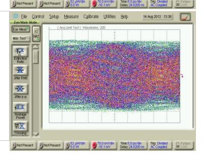
Reflection correction using 8-tap filter
