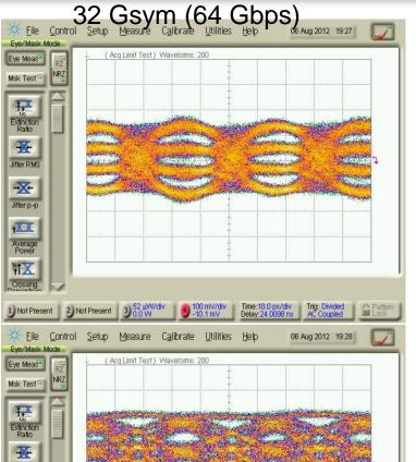
Reflection correction using 8-tap filter
