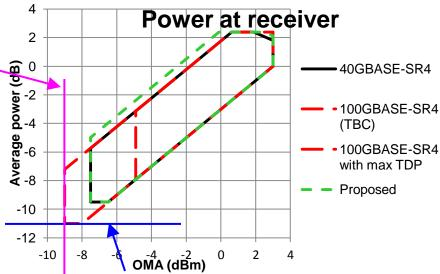
Any signal below the blue line is not compliant. Signal detect should be allowed to flag it (SIGNAL\_DETECT = FAIL)
