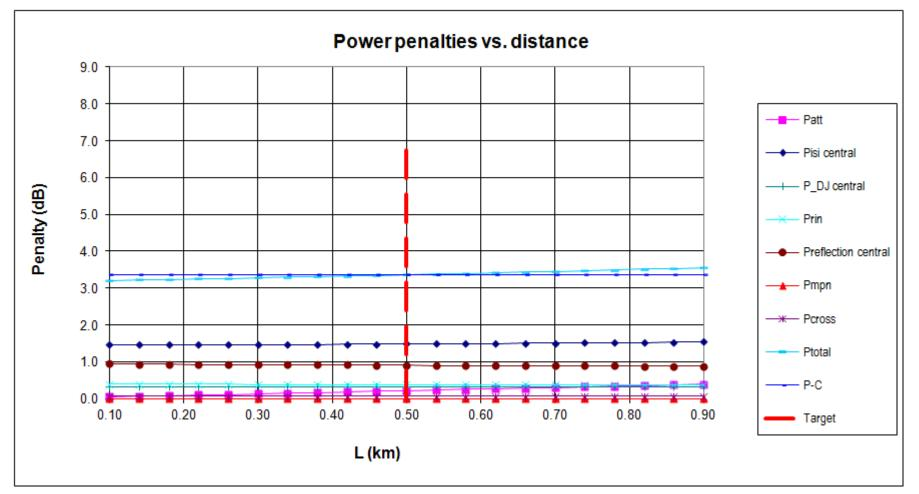
The above chart is taken from the tab Base of the updated Example PSM Link Model. It does not explicitly show the power required for the target TP4 eye opening, Peye, but distributes the penalty in other power penalties. For this example, Peye at 500 m equals 0.38 dB.
