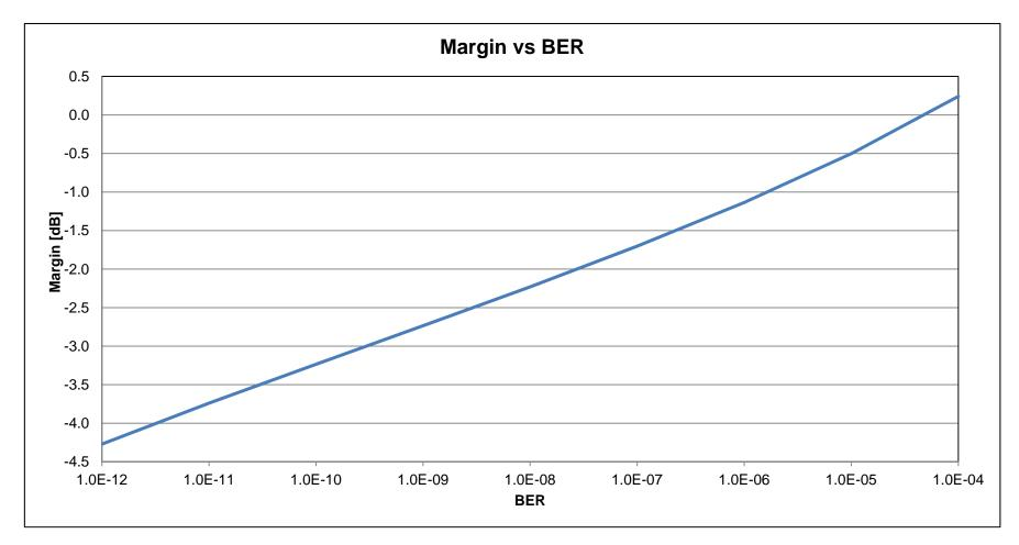
The above chart shows the benefit to an optical link from FEC. Operating at a higher BER not only appears to improve the Rx sensitivity but all the noise related penalties are reduced as is the power required to open the eye to a target width. For 100G PSM4, capturing all the benefit of KR4 FEC enhances the link margin by ~4.3 dB when compared to operating at a BER =  $10^{-12}$  without FEC.
