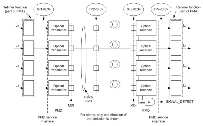
• TP1 and TP4, shown here for illustration only, represent the start and end of link budget calculations. They may not be accessible points for measurements, nor are they intended as reference points for specifications.
