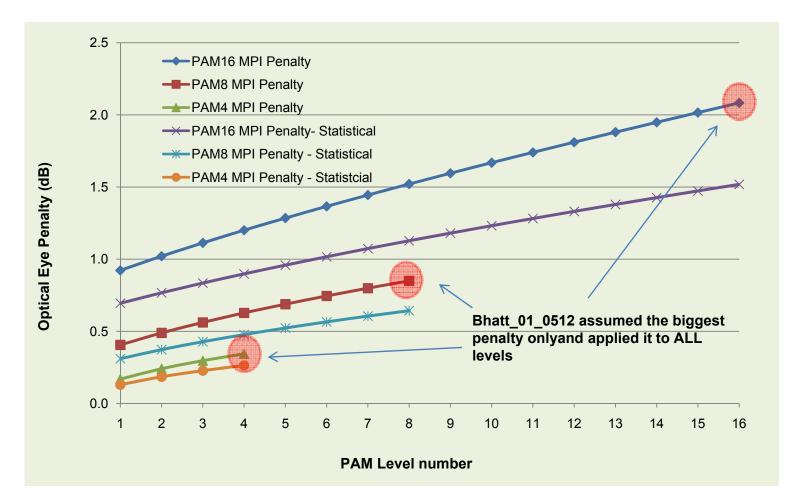
Using R<sub>ROSA</sub>=R<sub>TOSA</sub>=R<sub>Conn</sub>=-35dB ,4 connectors and 6dB ER, the table below shows the **maximum** statistical upper bound MPI penalty compared to Bhatt\_01\_0512 Upper Bound method MPI penalty
