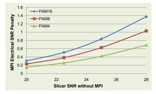
• As shown in the above graph, if the Slicer SNR was 20dB before MPI, with MPI if will be reduced by **0.15dB to 0.3dB** as a function of PAM modulation order. This is a manageable penalty.
