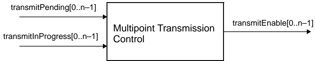
Figure 103–4—Multipoint Transmission Control service interfaces
