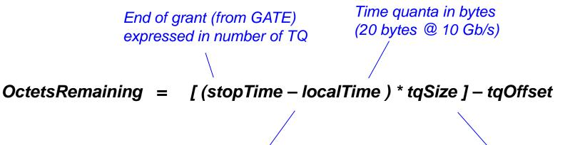
The variable holds the value of the local timer used to control MPCP operation. This variable is advanced by a timer at 62.5 MHz and counts in TQ and it is reloaded at ONU with the received timestamp value (from OLT). This variable denotes the offset (in octet times) of the current actual time from the localTime variable (which maintain the current time in units of TQ)
