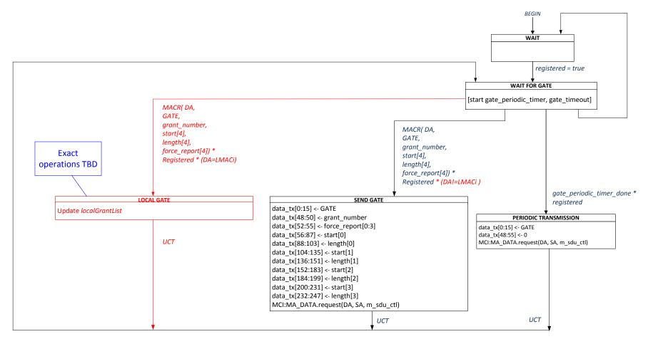
Note: new variables/constants<br/>introduced by these changes<br/>need to be reflected in the<br/>corresponding sections tooState machine derived by extending<br/>state machine defined in Figure 77-<br/>28 (Gate Processing state diagram<br/>at OLT) from clause 77.3.5.6
