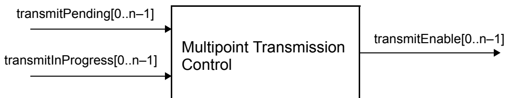
Figure 103-5—Multipoint Transmission Control service interfaces
