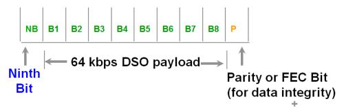
8 Payload bits + NBS + Parity bit = 10 bit DSO format
