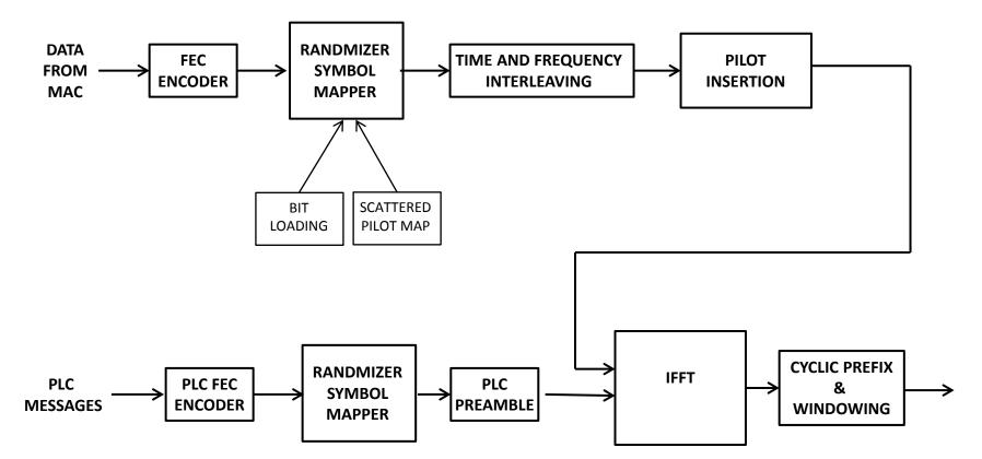
EPoC Downstream Transmitter Block Diagram (starting point)
