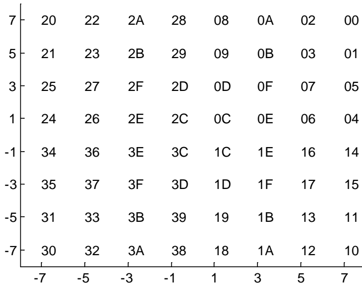
Figure 1–23 - 64-QAM Constellation Mapping of \{y_{i,0}y_{i,1}y_{i,2}y_{i,3}y_{i,4}y_{i,5}\}
