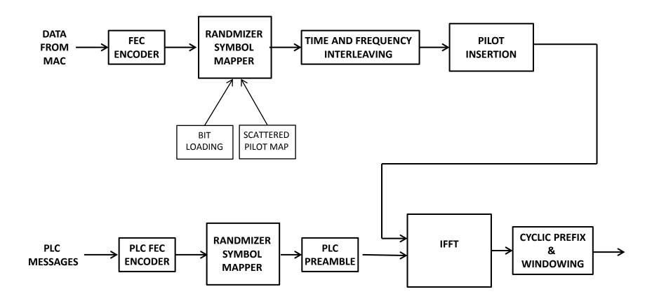
**EPoC Downstream Transmitter Block Diagram (starting point)**
