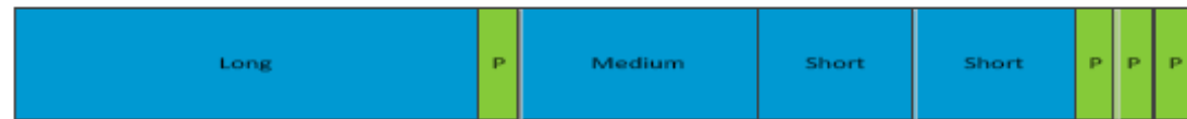
Option 2 – Parity follows info except of last 2-3 codewords Info of all codewords transmitted following Parity and CRC of all codewords
