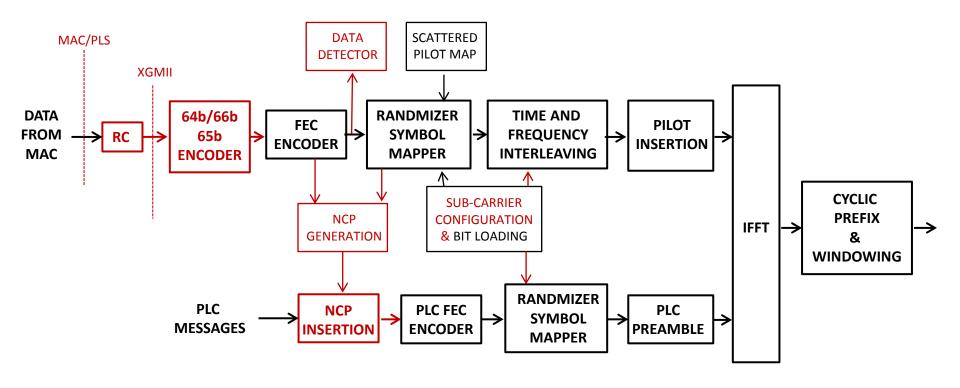
EPoC Downstream CLT Transmitter Block Diagram
