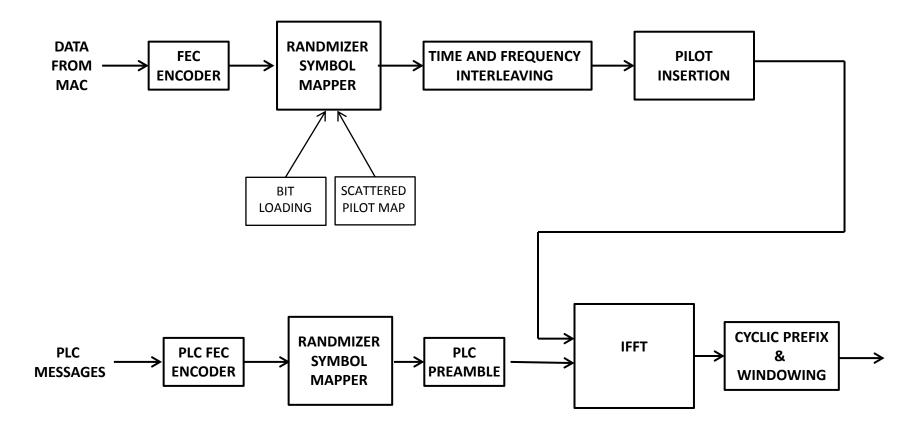
**EPoC Downstream Transmitter Block Diagram (starting point)**
