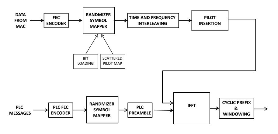
**EPoC Downstream Transmitter Block Diagram (starting point)**
