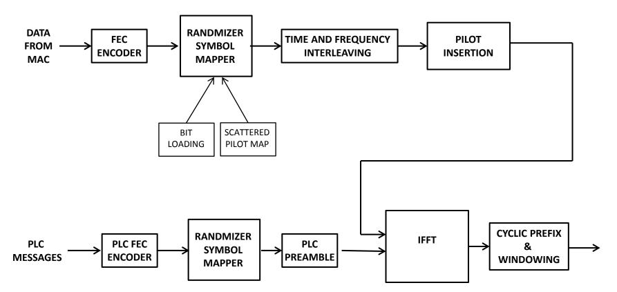
EPoC Downstream Transmitter Block Diagram (starting point)
