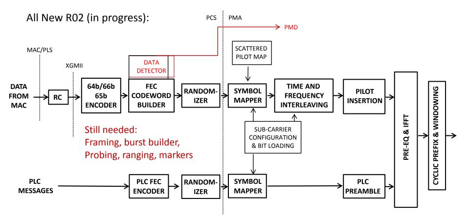
Assumption: Upstream PLC will be similar to downstream, with added functionality to control bursts separate from data
