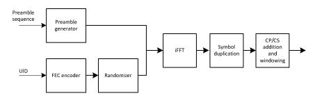
Figure 7-20 - Block Diagram of Initial Ranging Transmitter Processing
