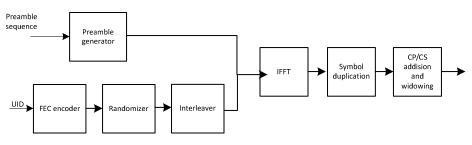
Figure 7–25 - Fine Ranging Transmitter Processing
