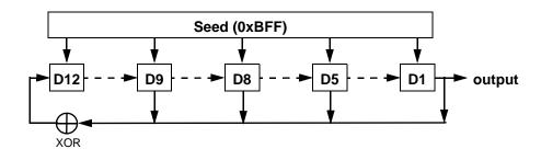
Figure 102–7—Probe sequence generator
