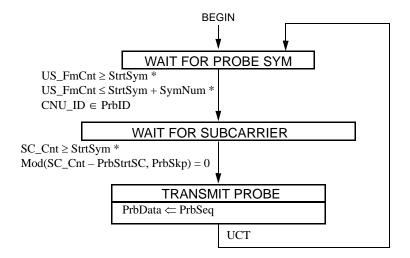
Figure 102-8—CNU Probe transmission control state diagram
