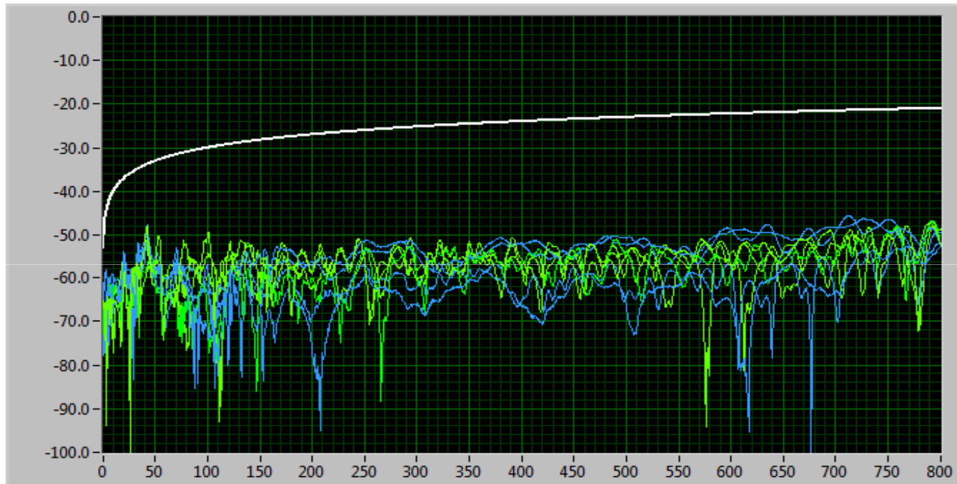
2-pair Cable to Cat-6A Cable TCL Spec
