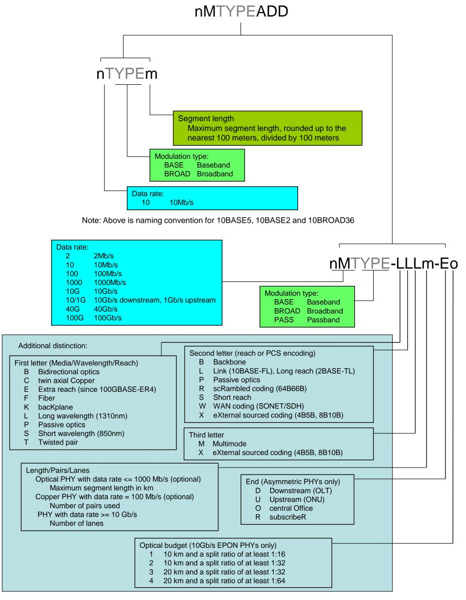
Note - The PCS and PMD family names are based on use of either the first or second letter. Examples are 10GBASE-L for 10Gb/s long wavelength PMD family and 10GBASE-R for 10Gb/s scrambled encoding PCS family.
