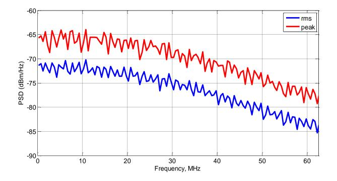
Peak PSD values measured for 1000BASE-T in test mode 4 (PAM5 with 11bit scrambler) on 100KHz RBW are seen larger than rms by less than 10dB. Sequence period is less than 1/100KHz and therefore the rms curve is not smooth as previous plots.
