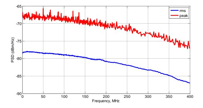
Peak PSD values measured for 10GBASE-T in test mode 1 (PAM2 with no THP) and on 100KHz RBW are seen larger than rms by more than 10dB. This mode uses PRBS 33 training pattern (33bit scrambler).
