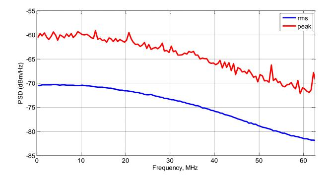
Peak PSD values measured for 1000BASE-T in forced master mode (PAM3 with 33bit scrambler) on 100KHz RBW are seen larger than rms by more than 10dB.
