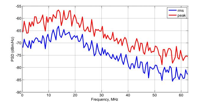
Peak PSD values measured for 100BASE-TX (MLT-3 with 11bit scrambler) on 100KHz RBW are seen larger than rms by less than 10dB. Sequence period is less than 1/100KHz and therefore the rms curve is not smooth.
