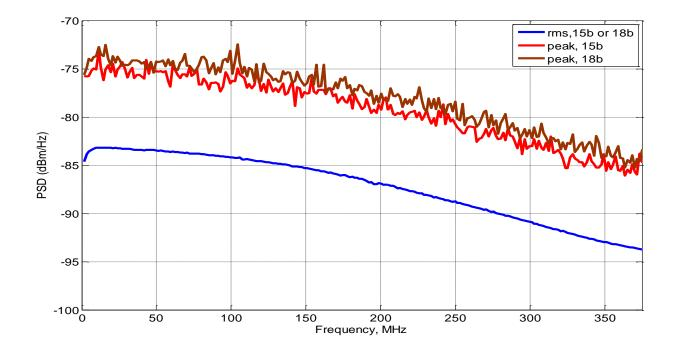
Peak PSD values measured for a signal generated by AWG with 2D-PAM3 modulation and 18bit scrambler. Symbol rate is 750Msps and (0.75+0.25Z<sup>-1</sup>) PRF is used. Measured peak values on 100KHz RBW are seen larger than those for 15bit scrambler.
