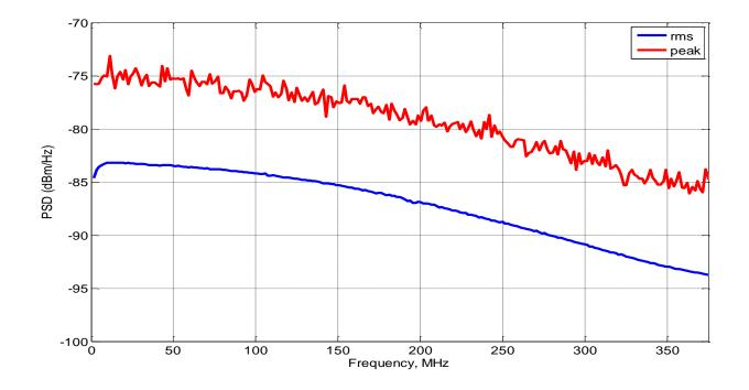
Peak PSD values measured for a signal generated by AWG with 2D-PAM3 modulation and 15bit scrambler. Symbol rate is 750Msps and (0.75+0.25Z<sup>-1</sup>) PRF is used. Measured peak values on 100KHz RBW are seen larger than rms by about10dB.
