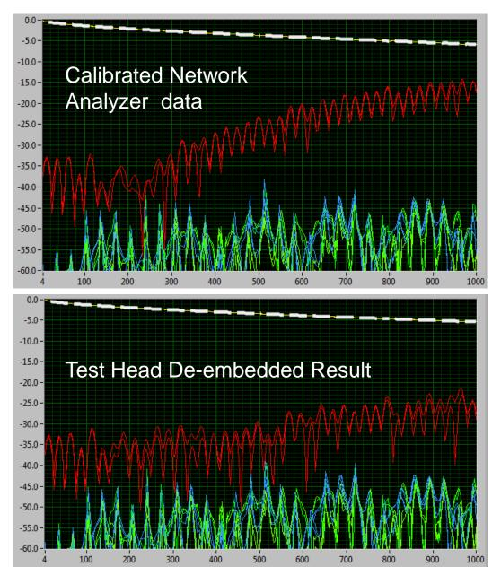
Test Head De-embedding provides high accuracy for 4 port Network Analyzer data
