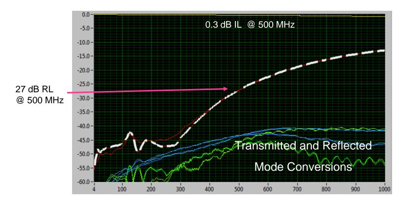
Mixed Mode plots  $Z_{DM} = 100\Omega$   $Z_{CM} = 25\Omega$
