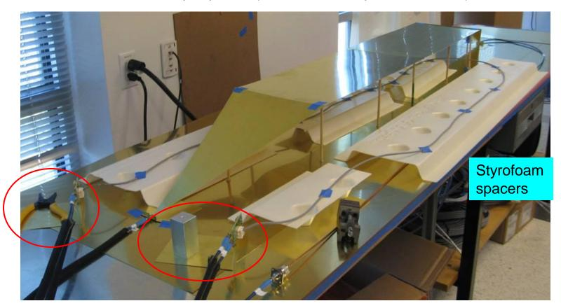
A small weight (block and pliers in this case) stabilizes the head positions and provides good electrical reference contact if metals are not tarnished.
