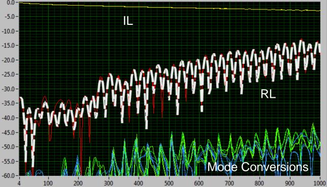
Typical 1 pair cable laid out and back 4 cm over the reference plane between near end and far end port pairs (note: the EMC stripline is not in use)
