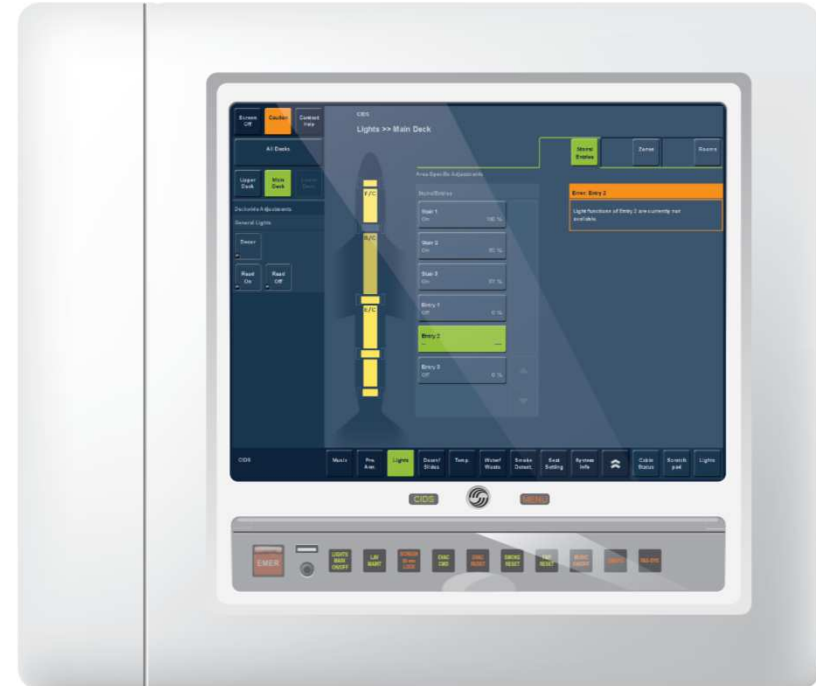
The Airbus Flight Attendant Panel (FAP) is a multi-domain device.
