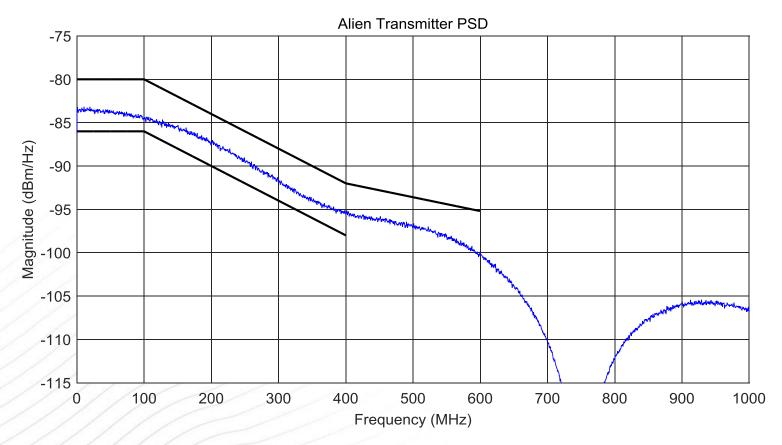
Assumed Alien Transmitters compliant with 1000BASE-T1 PSD limit
