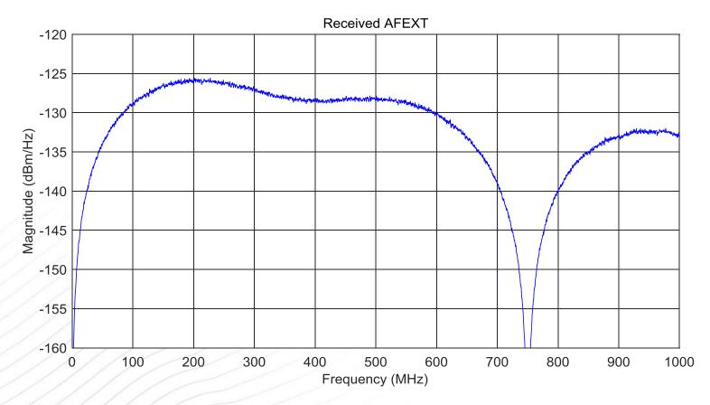
Computed based on Alien Transmitters PSD and AFEXT limit as per 97.5.6.3.4 in P8023bp-D2.1.pdf and assuming a worst case scenario with Alien disturbers having 2 m link segments. The AFEXT limit line is extrapolated beyond 600 MHz using same equation for this plot.
