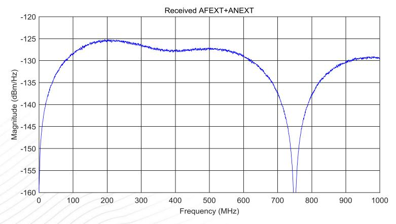
Computed based on Alien Transmitters PSD and ANEXT and AFEXT limits as per 97.5.6.3.2 and 97.5.6.3.4 in P8023bp-D2.1.pdf
