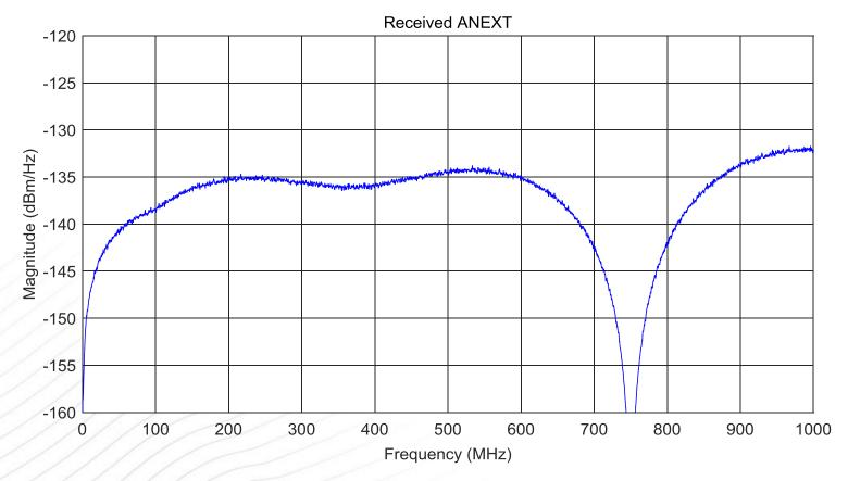
Computed based on Alien Transmitters PSD and ANEXT limit as per 97.5.6.3.2 in P8023bp-D2.1.pdf. The ANEXT limit line is extrapolated beyond 600 MHz using same equation for this plot.
