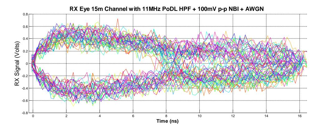
Eye closed: cannot detect 2<sup>nd</sup> part of bit cell
