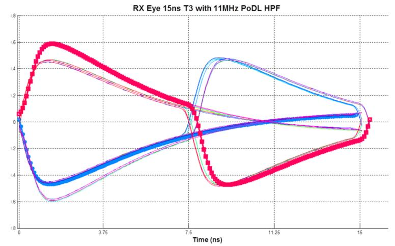
A 15ns T3, is more compatible with 100BASE-T1 channel and Baud rate. On the 1000T1 Channel with PoDL, a '1' symbol (absence of transition) is completely distorted. Even without noise, almost impossible to detect with a comparator receiver
