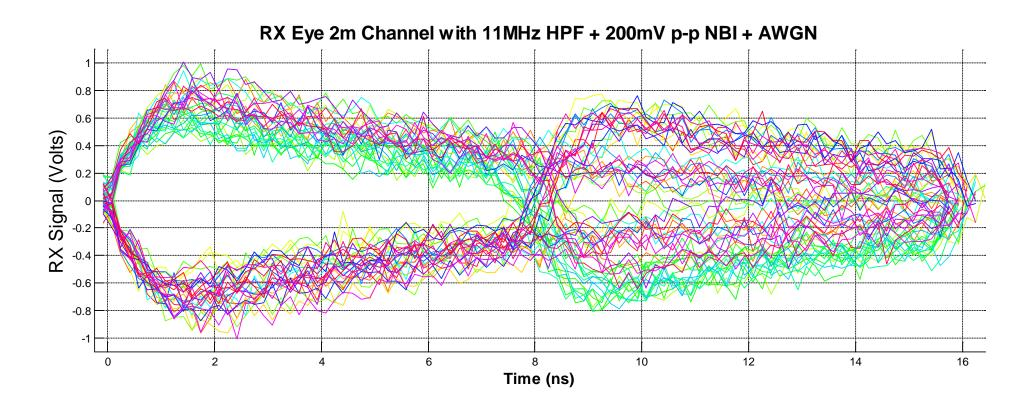
Eye closed: cannot detect 2<sup>nd</sup> part of bit cell
