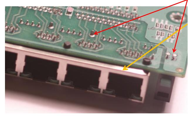
As shield connection fair, ground connection with a lot of coupling to signal path
