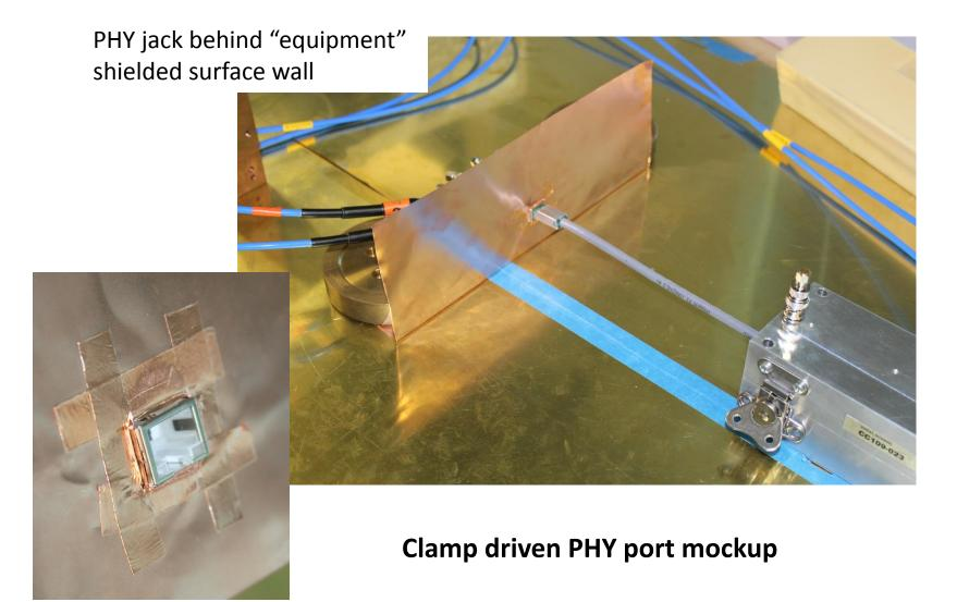
The bulk of the induced energy and field strength is in the 20 cm region directly in front of the PHY connection
