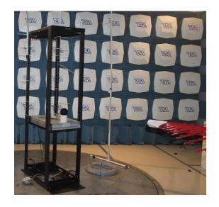
This is in many ways similar to a chamber EMC test where the radiating antennae is directly in front of the equipment port
