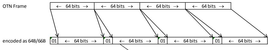
Use the Ethernet Stack to stripe and FEC encode the OTN frame when carrying over an Ethernet Module for an OTN IrDI or client interface
