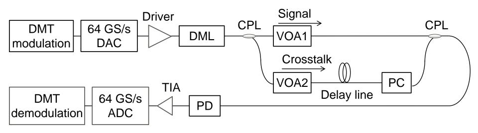
(DML: Directly modulated laser, VOA: Variable optical attenuator, CPL: Coupler, PC: Polarization controller, TIA: Trans-impedance amplifier)
