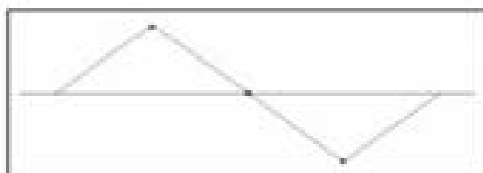
Figure 5.1. Correct timing: e_n = (-1 - 1) \cdot 0 = 0 .
