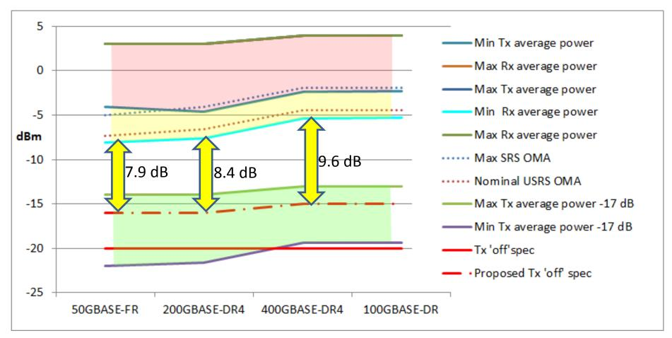
20 dB min extinction from modulator would allow 17 dB reduction in average Tx power Meeting Tx 'off' spec relies on controlling lane to lane Tx average power per lane
