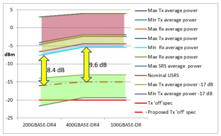
20dB min extinction from modulator would allow 17 dB reduction in average Tx power Meeting proposed Tx 'off' spec relies on controlling lane to lane Tx average power variation
