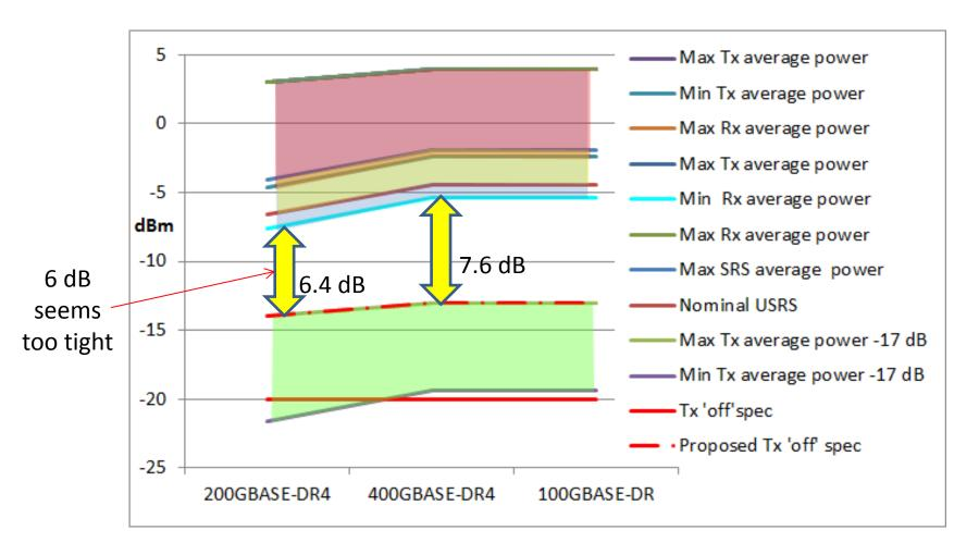
20 dB min extinction from modulator would allow 17 dB reduction in average Tx power
