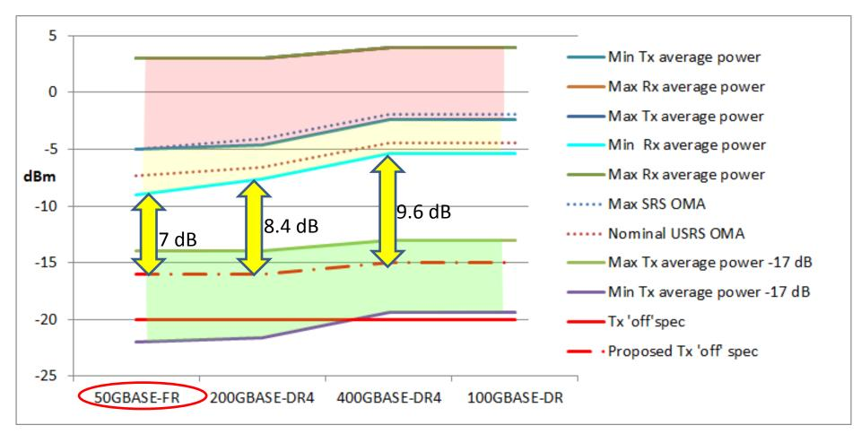
20 dB min extinction from modulator would allow 17 dB reduction in average Tx power Meeting Tx 'off' spec relies on controlling lane to lane Tx average power per lane very closely
