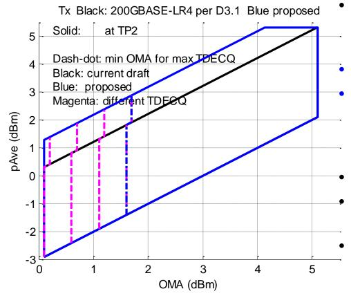
A single Tx waveform measurement is used to find TDECQ, OMA, mean power, and extinction ratio Black polygon (partly hidden under blue one): Tx spec in D3.1, with 4.5 dB min. extinction ratio
