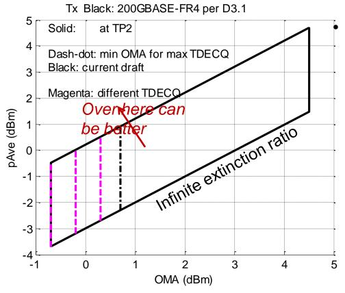
Black polygon: Tx spec in D3.1, with 4.5 dB min. extinction ratio
