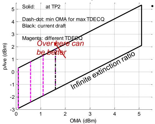
Black polygon: Tx spec in D3.1, with 4.5 dB min. extinction ratio
