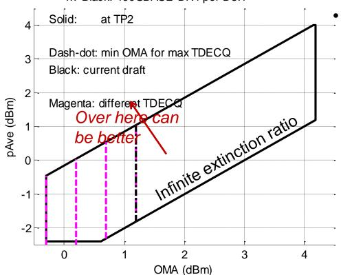
Black polygon: Tx spec in D3.1, with 5 dB min. extinction ratio
