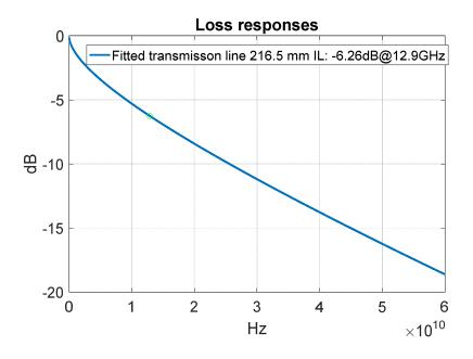
216.6 mm of fitted transmission line is 6.26 dB at 12.98Ghz as require for COM
