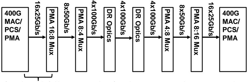
Constrained routing/pairing: Opt 1, constrained PCB routing that keeps natural pairs together. Opt 2, Arbitrary routing on PCB possible if using a programmable lane Swizzle in MAC/PCS/PMA
