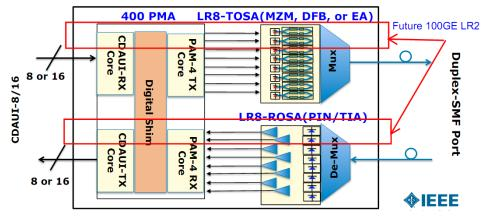
400GBASE-LR8 use 8:1 optical Mux/DeMux@3.5dB, while 100GbE use 2:1 optical Mux/Demux@1.5dB. This difference should be included in Breakout 100GE PMDs.
