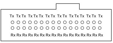
400GBASE-SR16 optical lane assignments for the MDI receptacle when viewed looking into the receptacle with keyway feature on top.
