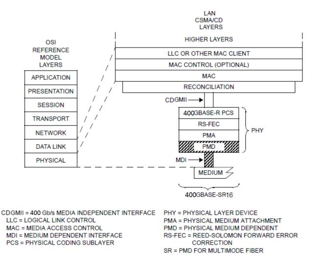
Editor's note: The RS-FEC layer may be merged into 400GBASE-R PCS layer, depending on the choice of architecture by the Task Force.
