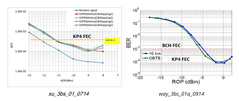
A BER floor that close to the FEC operation point, even under "ideal" laboratory conditions, will certainly lead to unstable performance in the field under practical field conditions
