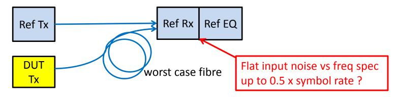
SRS test source metric: BER measurement based (but without worst case fibre), using reference Rx and reference EQ; DUT Tx and fibre is replaced by the SRS test source.
