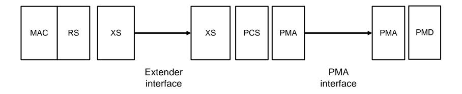
XS and extender interface is used to extend the xMII so that the raw data stream can be presented to the PCS
