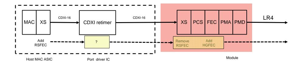
Complex module to handle coding & FEC in advance of host integration
