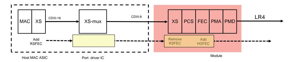
If RS-FEC is sufficient for 8x50 C2M, some form of mux function could change from CDXI-16 to CDXI-8
