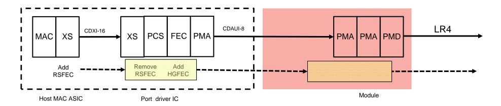
Alternate view could be allowed by the architecture, PMA mux function changes from CDAUI-8 to CDAUI-4
