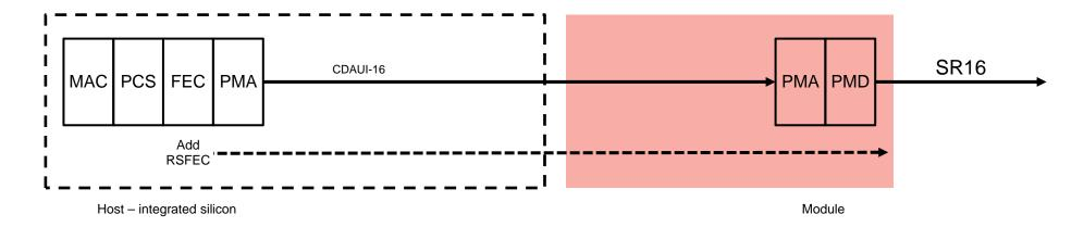
Driver integrated with host ASIC, indistinguishable from config #1 for external view
