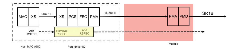
Definition for 16-bit XS & SR16 PCS/FEC/PMA should be as similar as possible so that driver IC has minimal logic
