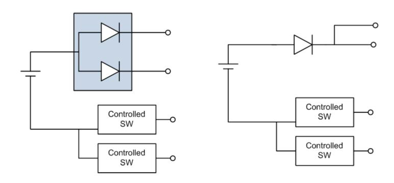
Vdiff is reduced by using single common diode or two matched diodes
