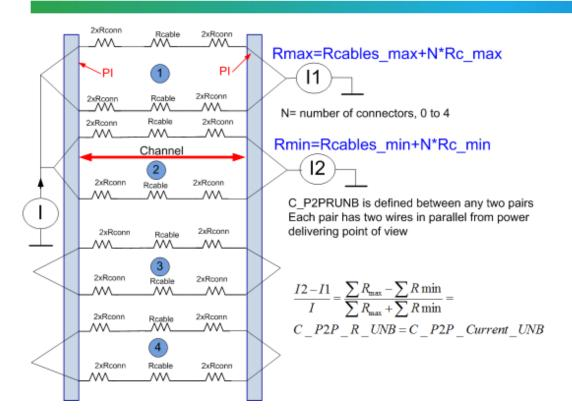
$Channel \_ P2P \_ Current \_ DIFFERENCE =$   $= I1 - I2 = I \cdot \frac{\sum R_{max}}{\sum R_{max}} - I \cdot \frac{\sum R_{min}}{\sum R_{min}} =$
