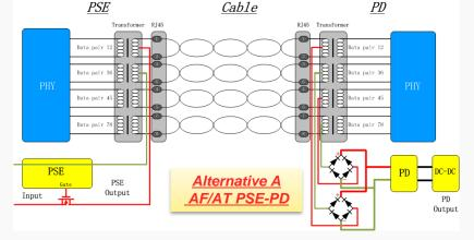
AF/AT PD shall be able to receive power from either 2-pair.
