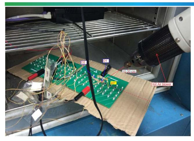
Figure 4 Narrow beam heat source
