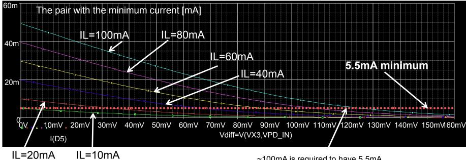
~100mA is required to have 5.5mA minimum over a pair with Vdiff=120mV.
