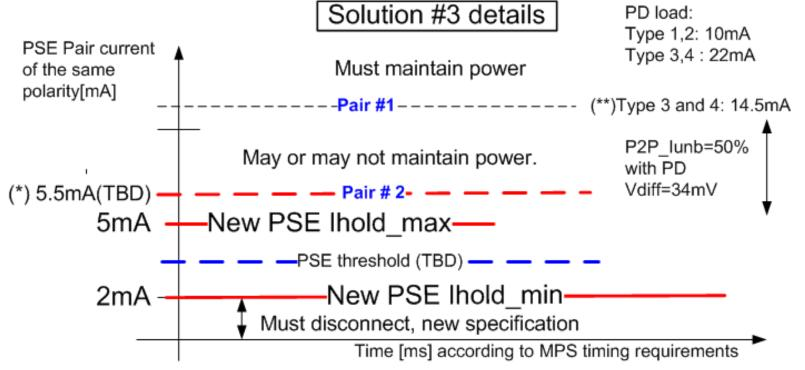
(\*) PD minimum guaranteed pair current with narrower Vdiff or minimum PD current over pair request (\*\*) P2P current distribution if we ask nothing from PD
