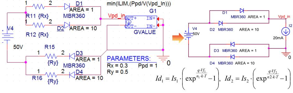
PD Diodes model and Vdiff at low and high current vs. E2EP2PCUNB. Yair Darshan , March 2015 Rev 008
