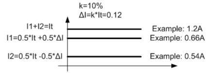
K\_i=(1+E2ECP2P\_C\_UNB\_i)/2. i=3,4. K3 and k4 are the equivalent (transformed) end to end channel P2P\_lunb for Type 3 and 4 systems.
