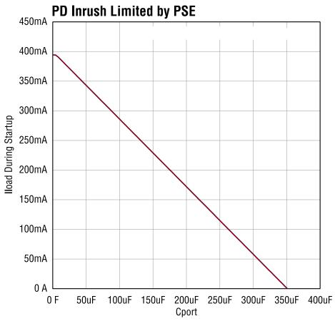
I<sub>load</sub> < [20mC – (C<sub>port</sub> \* 57V) ]/ 50ms
