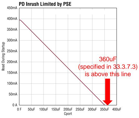
I<sub>load</sub> < [20mC – (C<sub>port</sub> \* 57V) ]/ 50ms
