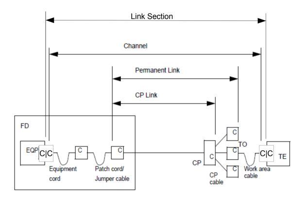
FD = floor distributor; EQP = equipment; C = connection (mated pair);
